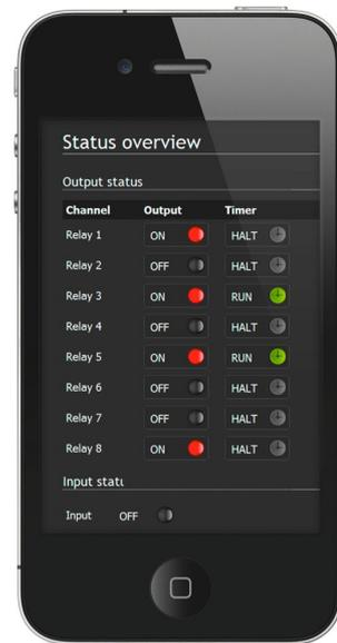
Operate the 8 relays using- your mobile device
